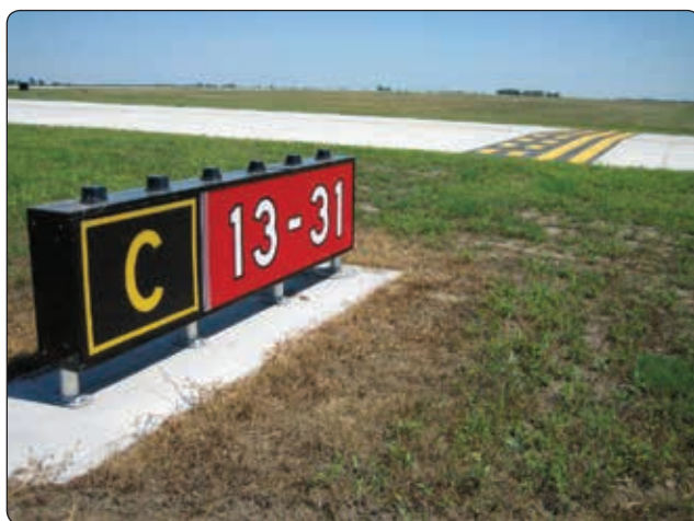
Figure 14-52. Runway 13-31 holding position sign and marking located on Taxiway Charlie.
