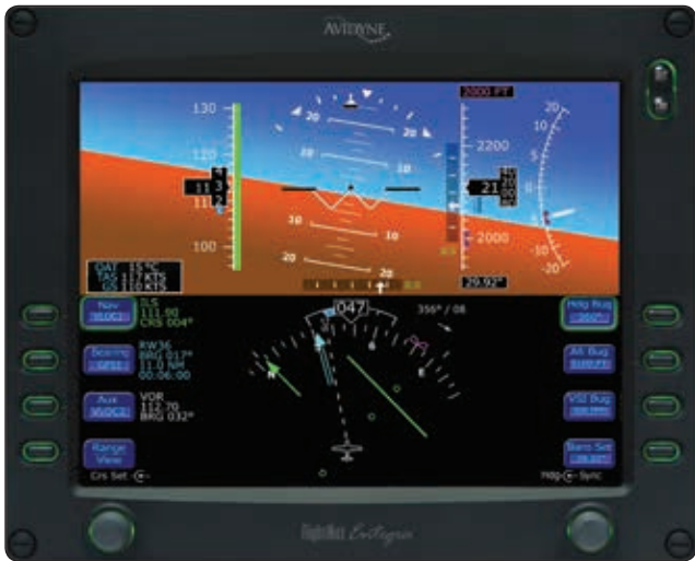
Figure 8-14. Chelton's FlightLogic (top) and Avidyne's Entegra (bottom) are examples of panel displays that are configurable.
