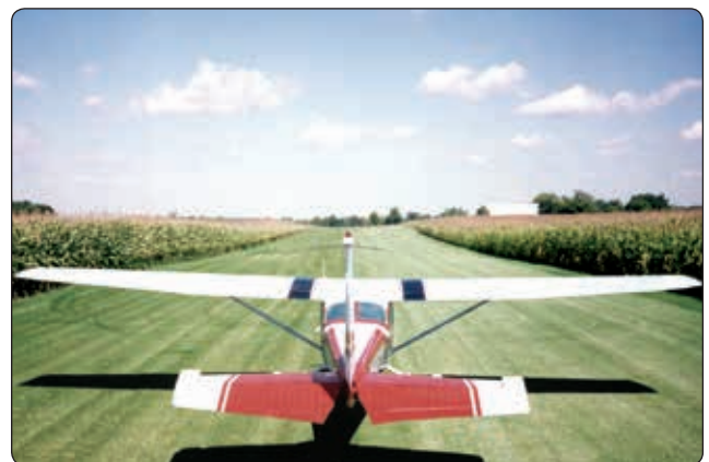
Figure 11-16. An aircraft's performance during takeoff depends greatly on the runway surface.
