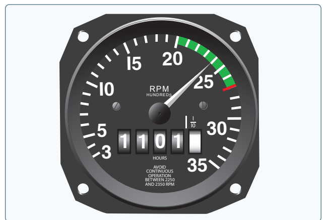
Figure 7-8. Engine rpm is indicated on the tachometer.
