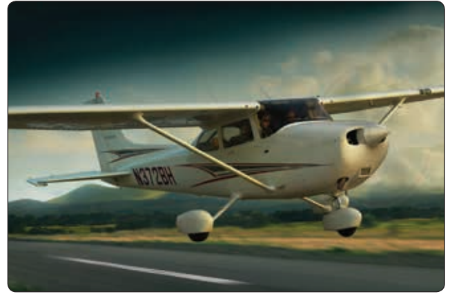
Figure 7-37. The landing gear supports the airplane during the takeoff run, landing, taxiing, and when parked.
