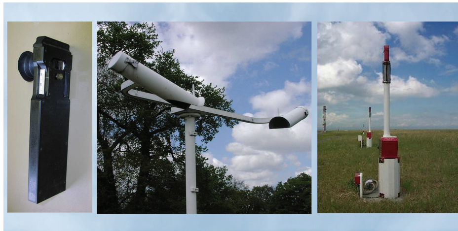
Figure 15.10: Gold's Visibility Meter, Visiometer and Transmissometer.
