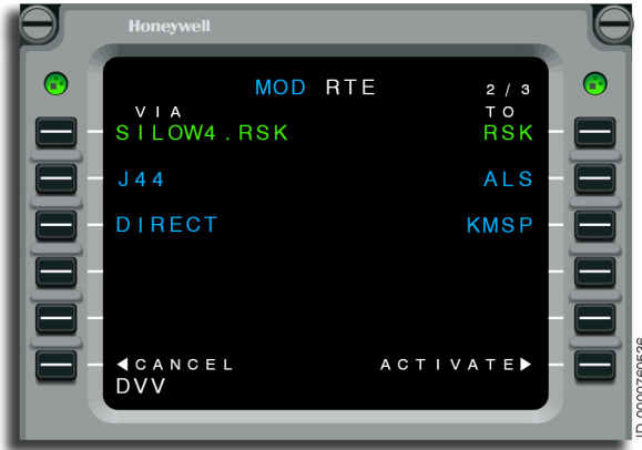
Figure 4-21 MOD RTE - DVV Entered in Scratchpad
