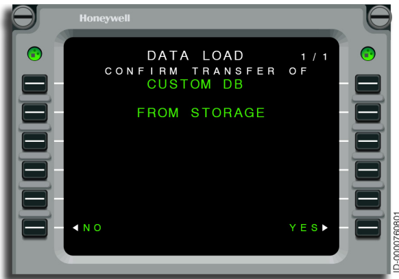
Figure 6-158 DATA LOAD - CONFIRM TRANSFER
