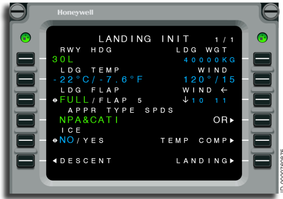
Figure 9-44 LANDING INIT - TEMP COMP
