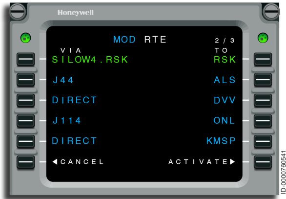
Figure 4-26 MOD RTE - ONL Loaded
