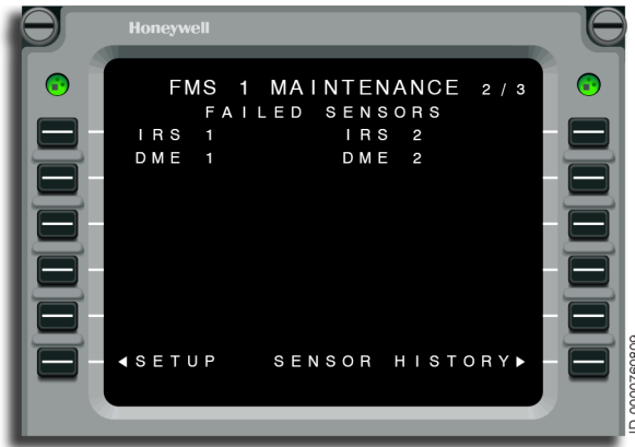
Figure 6-166 FMS 1 MAINTENANCE 2/3 - Setup
