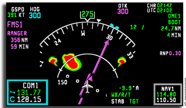
Figure 5-40 HSI Arc Mode With Weather
