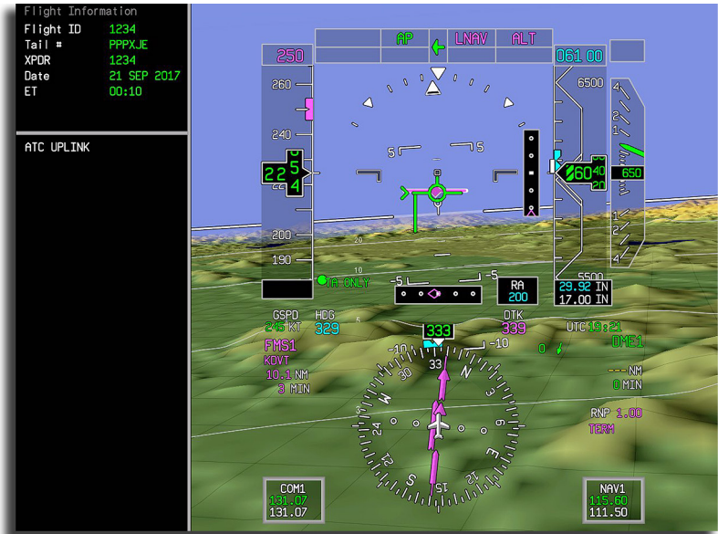
Figure 2-7 SVS on Pilot's PFD Window
