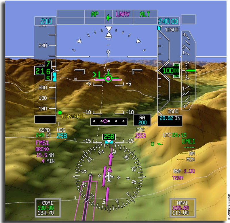
Figure 10-5 FMS LNAV Track Mode
