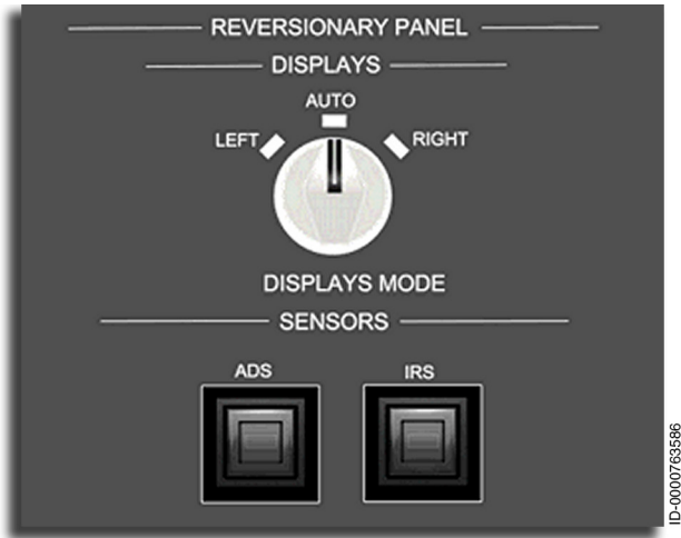
Figure 15-5 IRS REVERSIONARY PANEL
