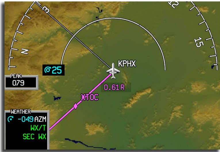
Figure 18-31 MFD With Specified Azimuth Select Line
