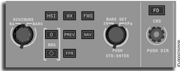
Figure 2-13 PFD Control Panel on Guidance Panel
