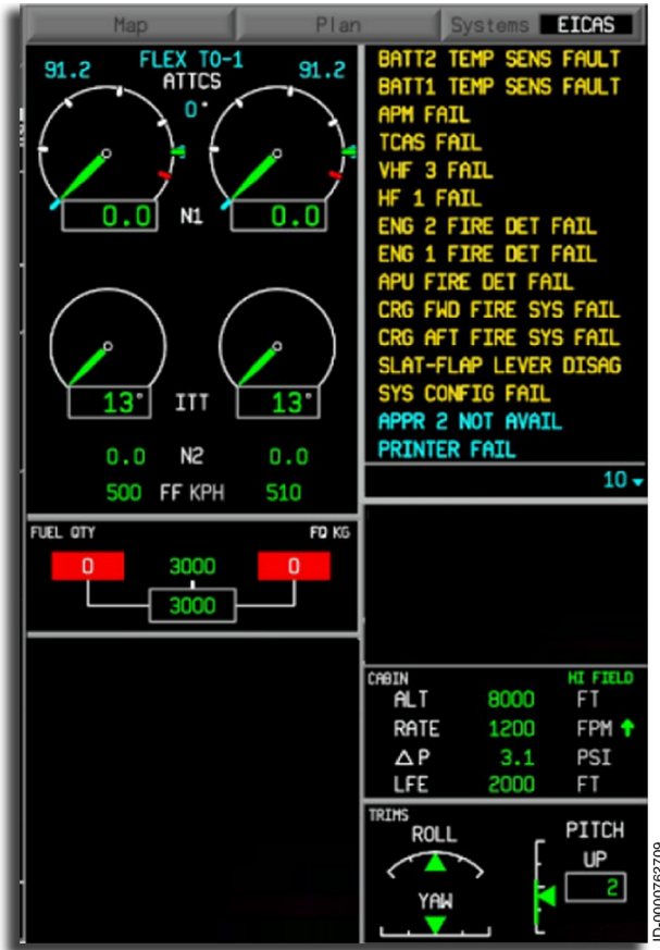
Figure 3-15 EICAS in Declutter Mode
