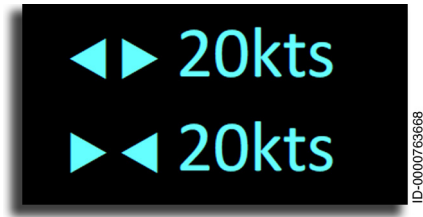
Figure 19-14 CDTI Closure Rate Display
