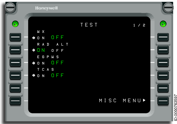
Figure 17-2 MCDU TEST Page With Radio Altitude Self-Test
