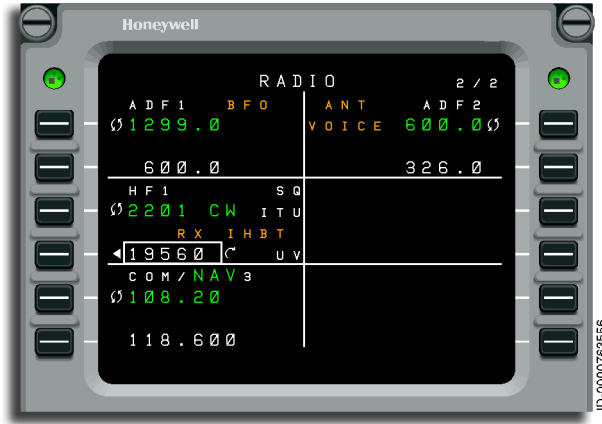
Figure 13-39 Amber Radio Indications
