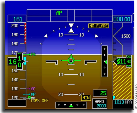
Figure 5-31 PFD with NO FLARE Annunciator
