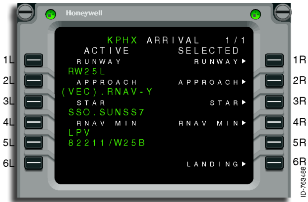
Figure 10-42 RNAV Approach With LPV Minimums Selected
