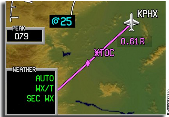
Figure 18-4 MFD Mode Annunciator Box
