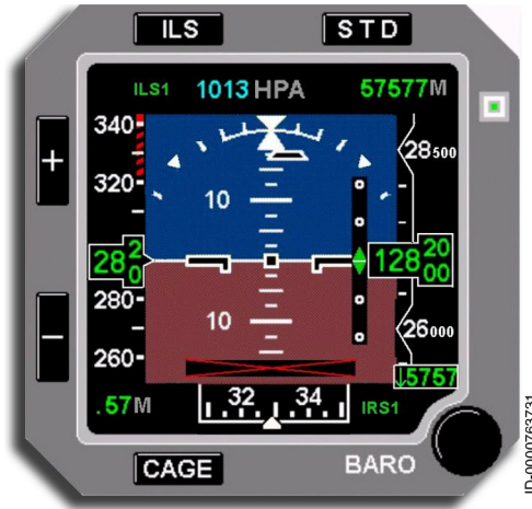
Figure 23-2 Integrated Electronic Standby (IES)
