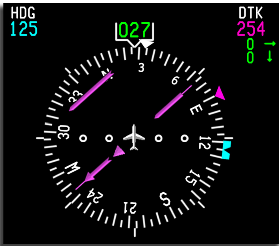
Figure 5-36 FMS Track Target Indicator
