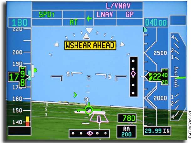
Figure 18-36 Predictive Windshear Caution Annunciator on the ADI
