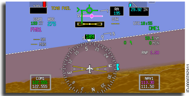
Figure 5-50 SVS With Ground Veil Overlay
