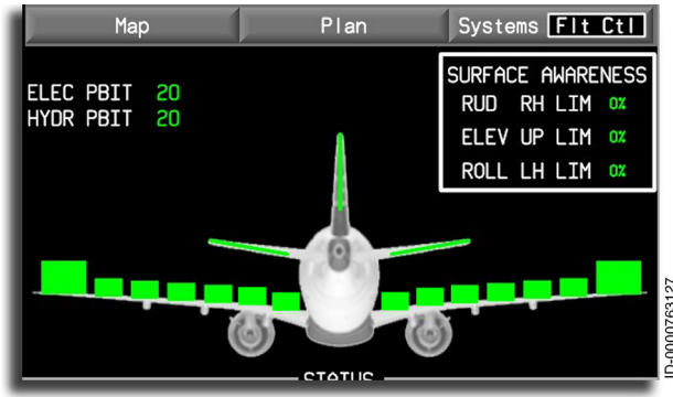
Figure 8-11 All Ground Spoilers Fully Deployed
