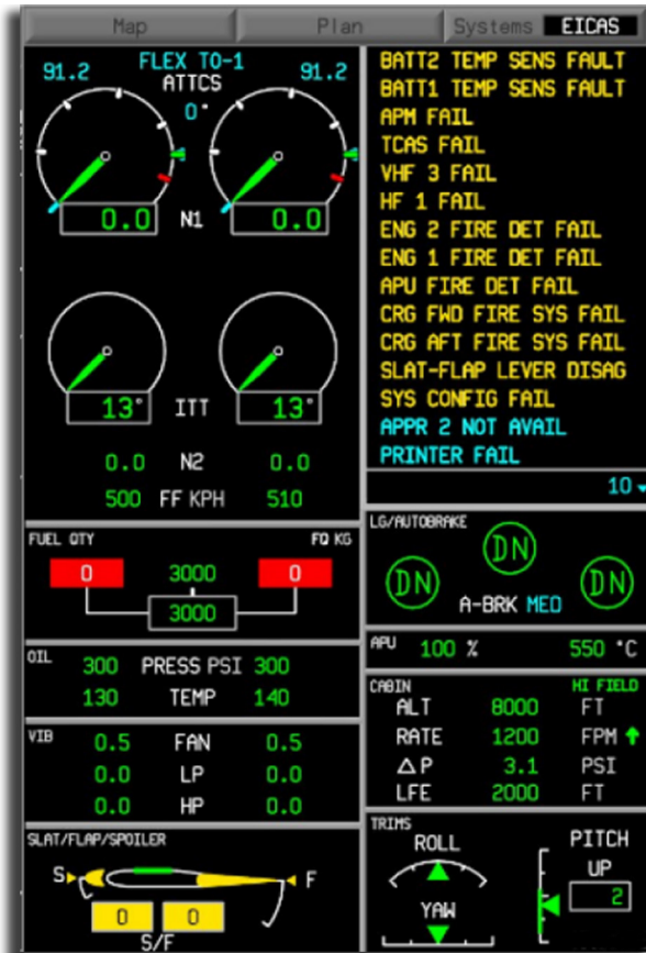
Figure 9-1 EICAS Window Functional Areas
