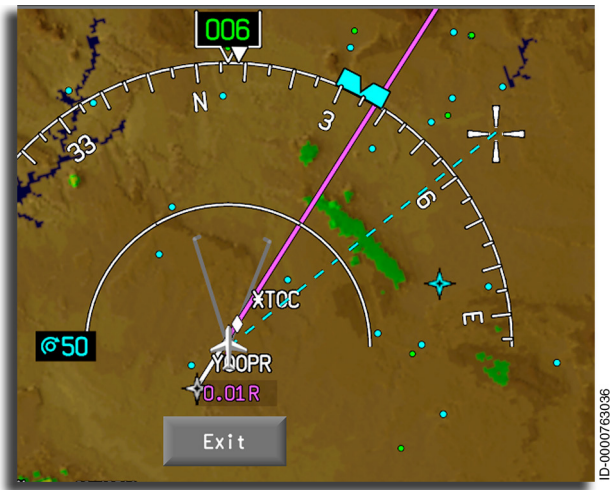
Figure 6-39 Designator Dashed Line From Intermediate Waypoint
