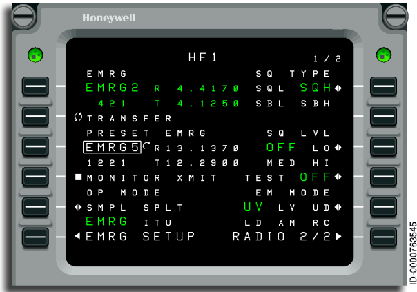
Figure 13-28 HF1 Emergency Mode Page
