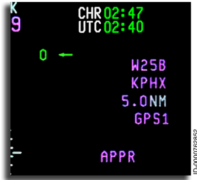
Figure 5-26 Reference Path Identifier
