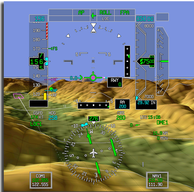
Figure 10-7 Localizer Mode Armed
