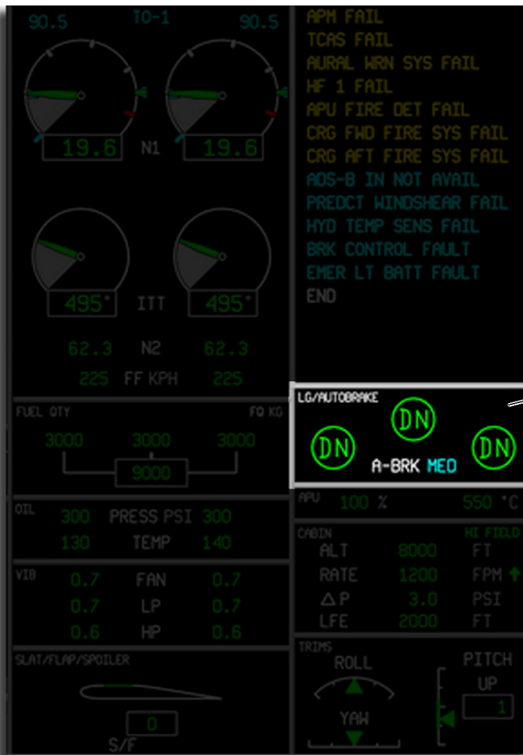
Figure 9-14 Landing Gear Status Location
