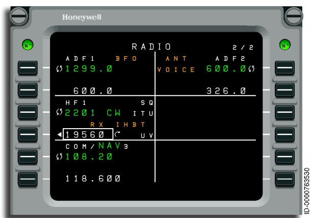
Figure 13-13 RADIO 2/2 Page Annunciators
