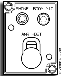
Figure 14-4 Observer Jack Panel
