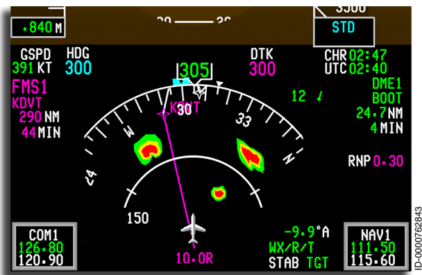
Figure 5-19 Lateral Deviation Display on PFD in Arc Mode With Map View
