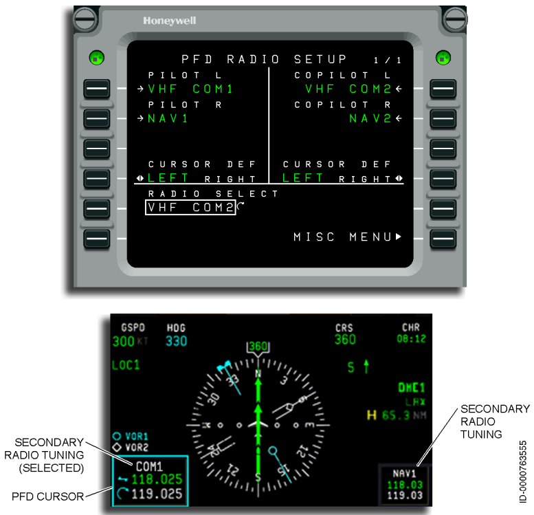
Figure 13-38 MCDU and PFD for Radio Setup
