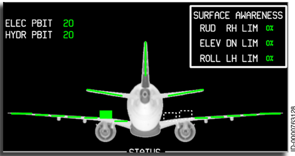
Figure 8-12 Abnormal Spoiler Displays
