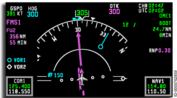
Figure 5-33 HSI Arc Mode
