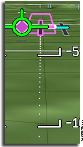
Figure 5-61 3D Extended Runway Centerline Classic
