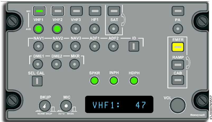
Figure 14-1 AV-900 Audio Panel With VHF3 and NAV3
