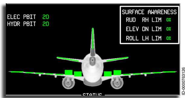
Figure 8-10 Ground Spoilers Deployed
