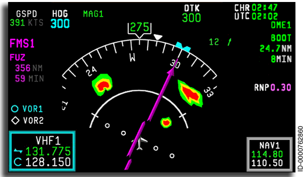
Figure 5-34 HSI Arc Mode With Weather Enabled
