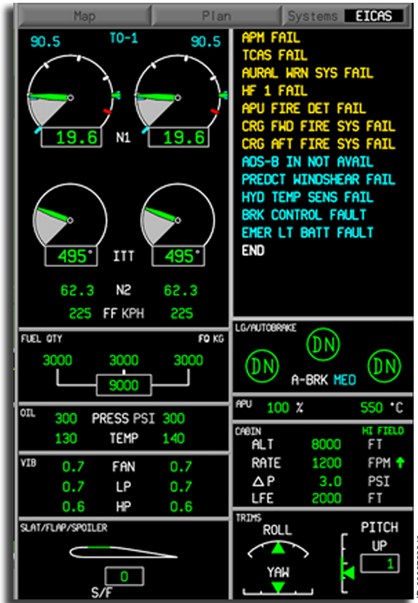
Figure 9-7 EICAS With FADEC On
