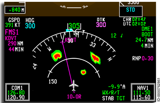
Figure 5-35 HSI Map Mode With Weather Enabled
