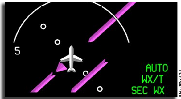
Figure 18-5 PFD Weather Annunciator Locations
