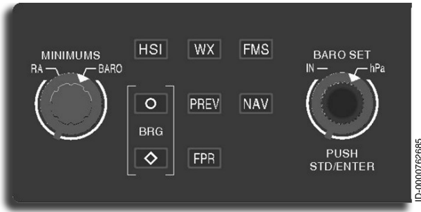
Figure 3-7 PFD Control Panel
