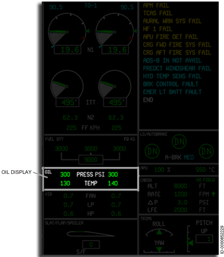
Figure 9-10 Engine Oil Readout Location
