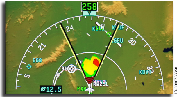
Figure 18-35 Predictive Windshear Display on the Lateral Map
