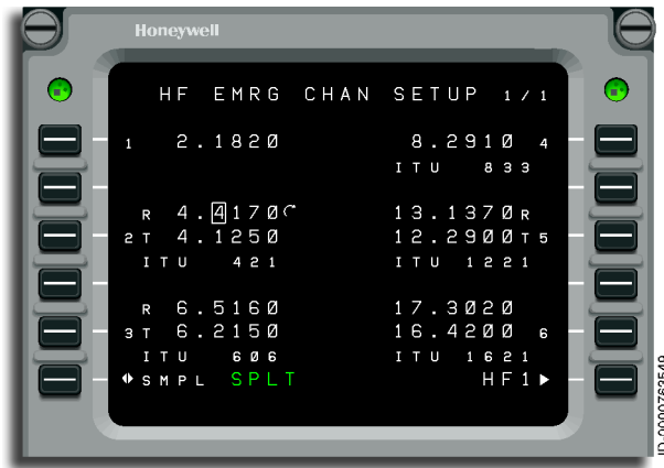
Figure 13-32 Emergency Channel Setup Page
