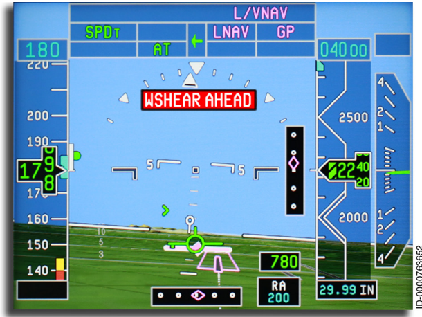
Figure 18-37 Predictive Windshear Warning Annunciator on the ADI
