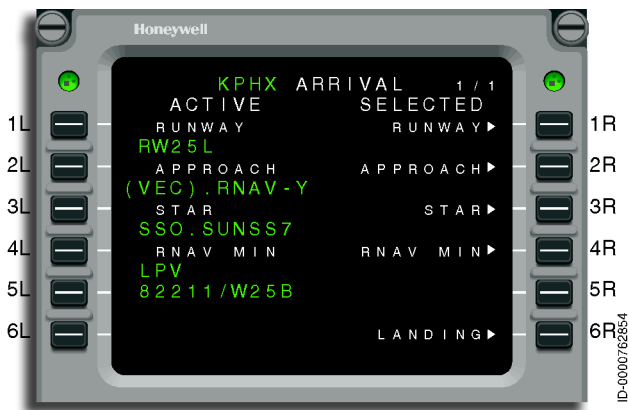
Figure 5-27 RNAV Approach With LPV Minimums Selected
