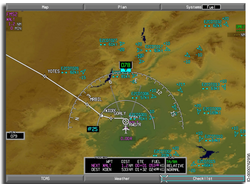
Figure 6-15 TCAS and CDTI Targets on INAV Display
