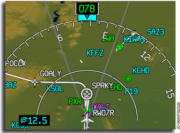
Figure 5-65 Field of View Lines
