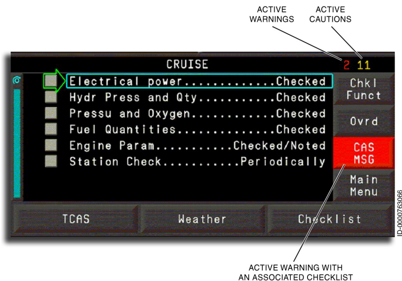
Figure 6-68 CAS Message Warnings and Cautions
