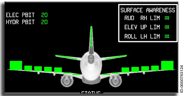
Figure 8-8 Speed Brakes Fully Deployed
