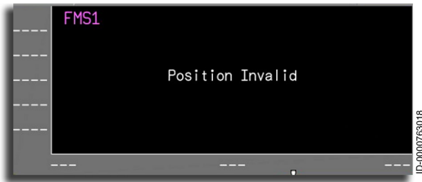
Figure 6-32 Vertical Position Invalid
