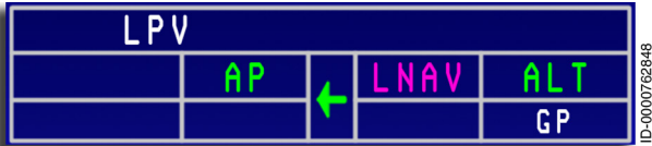
Figure 5-22 LPV Armed Indication
