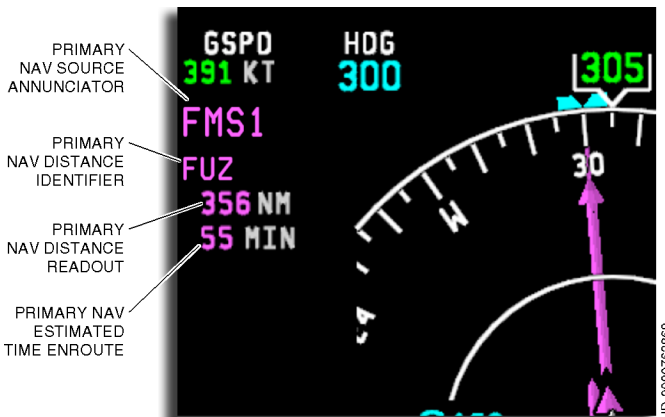
Figure 5-37 NAV and Heading Sources
