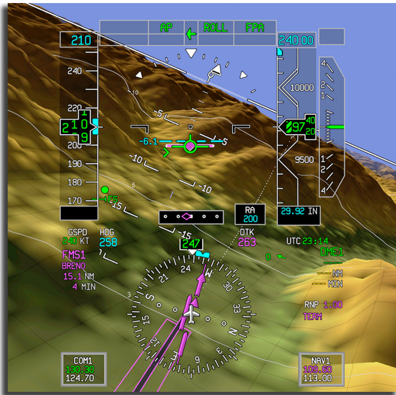
Figure 10-3 Roll Hold Mode
