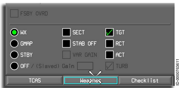
Figure 18-14 Primus 880 Weather Radar Controller
