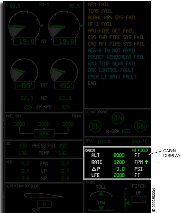
Figure 9-16 Cabin Pressurization Display
