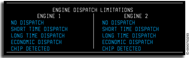
Figure 8-47 Engine Dispatch Limitations
