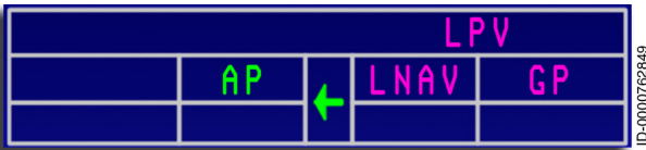
Figure 5-23 LPV Active Indication
