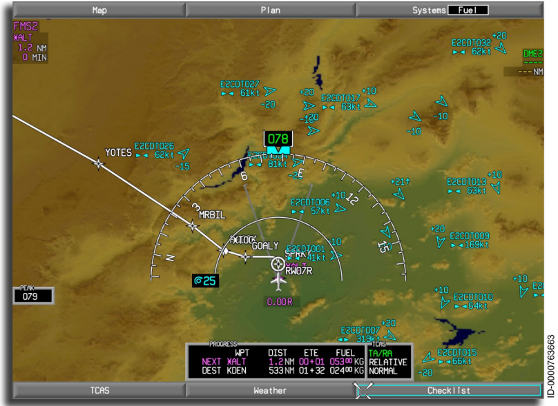
Figure 19-9 TCAS Targets Displayed on the MFD
