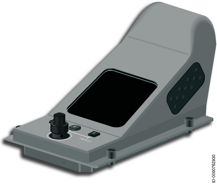
Figure 6-3 Controlling the MFD With the CCD
