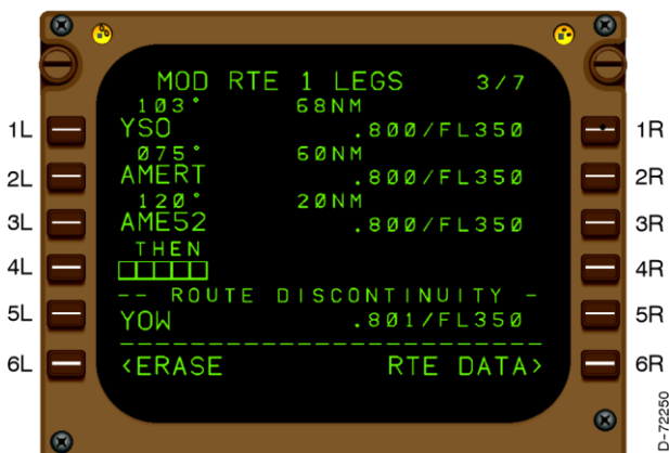
PB/D Waypoint in Route With Discontinuity Figure 11--5
