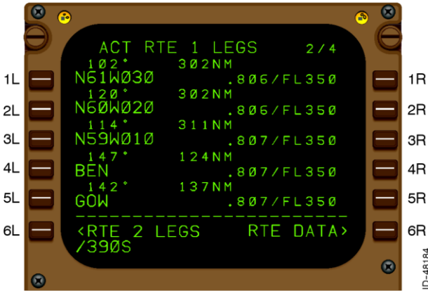
STEP CLIMB S/C Entry in Scratchpad Figure 6--26
