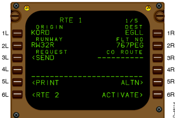
RTE 1 Route Entry Completed
