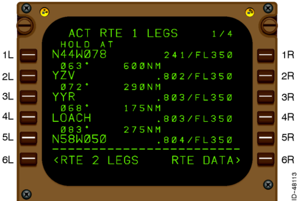
ROUTE DISCONTINUITY Cleared and Modified Route Activated Figure 4--
