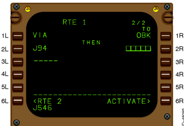
RTE 1 ROUTE ENTRY
