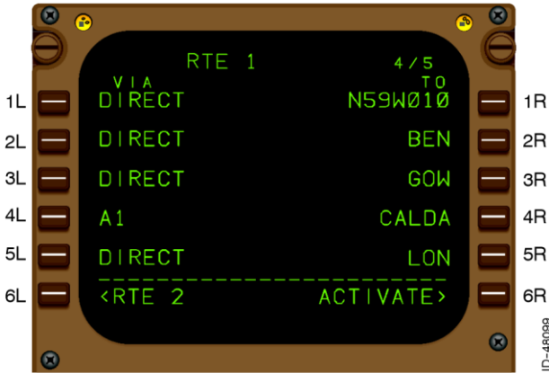
RTE 1 Route Entry Completed
