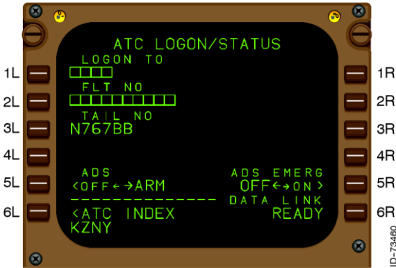
ATC LOGON/STATUS Page – ATC Facility ID
